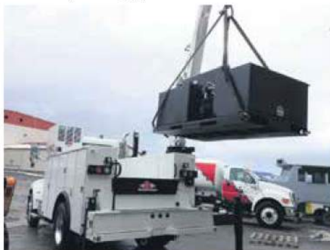
Lube skid is lifted onto the deck of a service truck.
